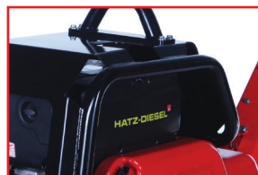
Central Lifting Hook for Easy Transportation
