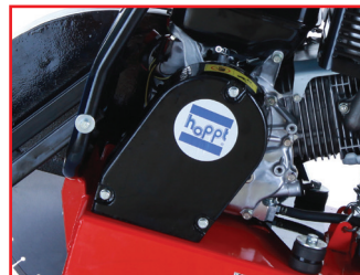
Belt Cover for Operators' Protection
